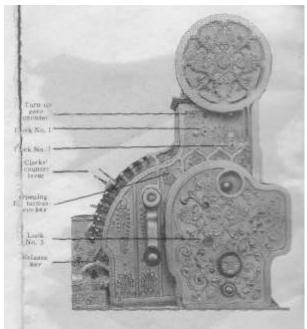
Text from top to bottom is: Turn to zero counter Lock No. 1 Lock No. 2 Clerks' counter lever Opening for turn to zero key Lock No. 5 Release key
